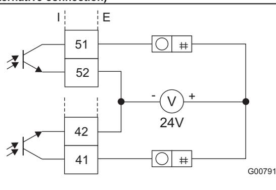
Digital input for external output switch-off or external totalizer reset
