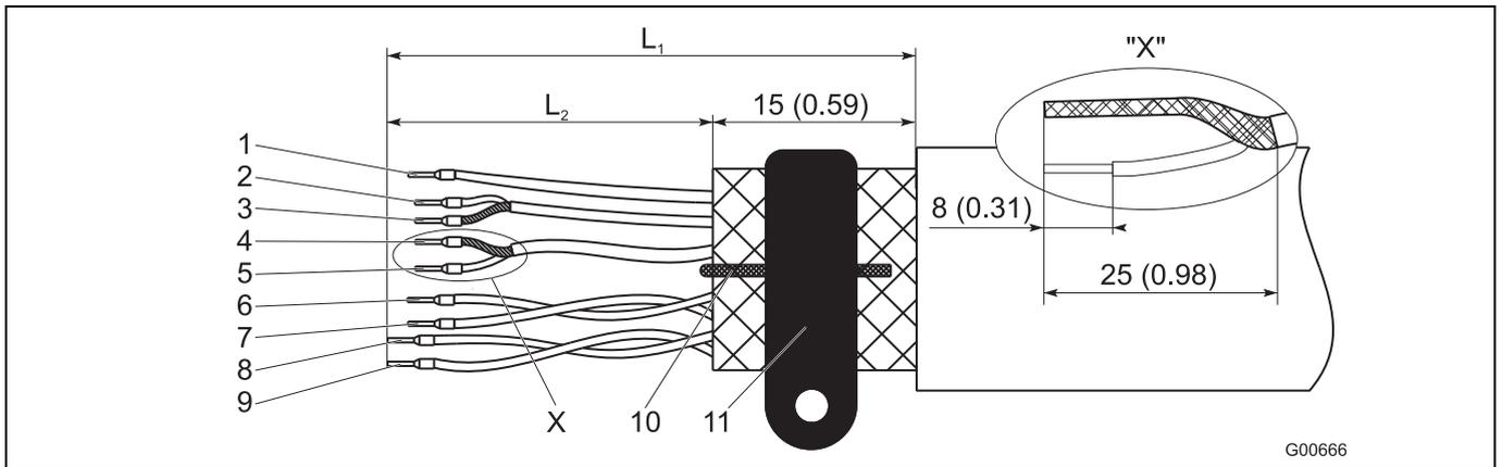
Fig. 33: Transmitter side, dimensions in mm (inch)
