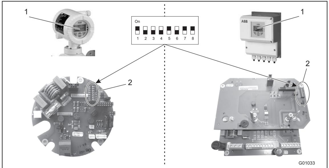
Fig. 56: Position of DIP switches
