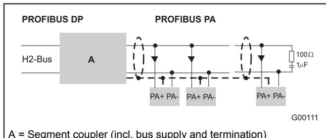
Fig. 52: Example for PROFIBUS PA interface connection
