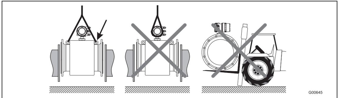
Fig. 8: Transport of flanged units larger than DN 400
