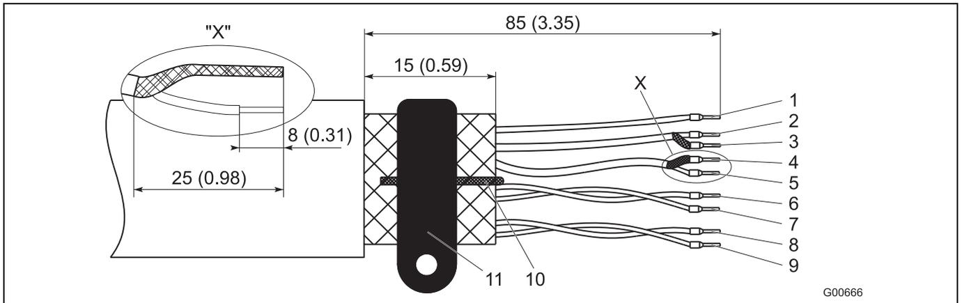
Fig. 32: Flowmeter sensor side, dimensions in mm (inch)
