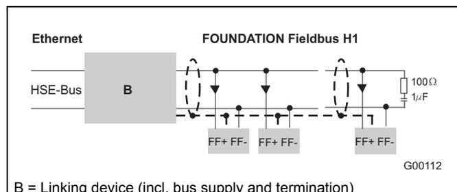
Fig. 53: Example for FOUNDATION Fieldbus interface connection
