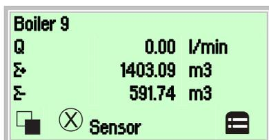
In the process display, a flow of zero flow is indicated, no flow measurement is performed.
