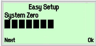
43. Use to start automatic adjustment of system zero.
