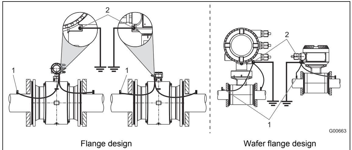
Fig. 26: Metal pipe, without liner
