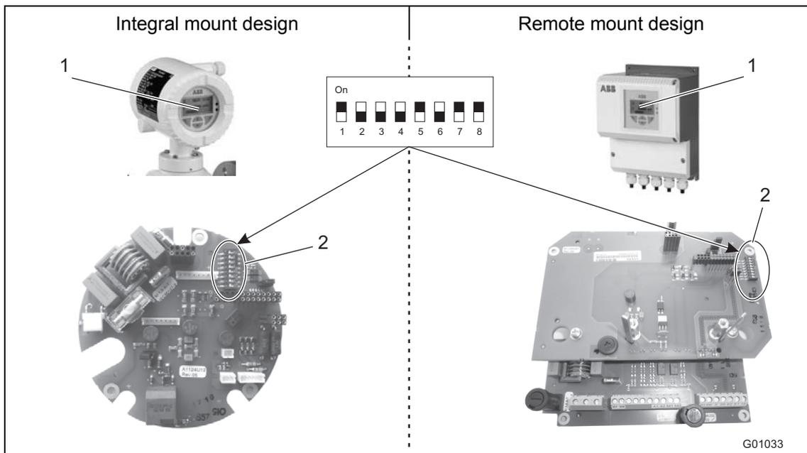
Fig. 55: Position of DIP switches
