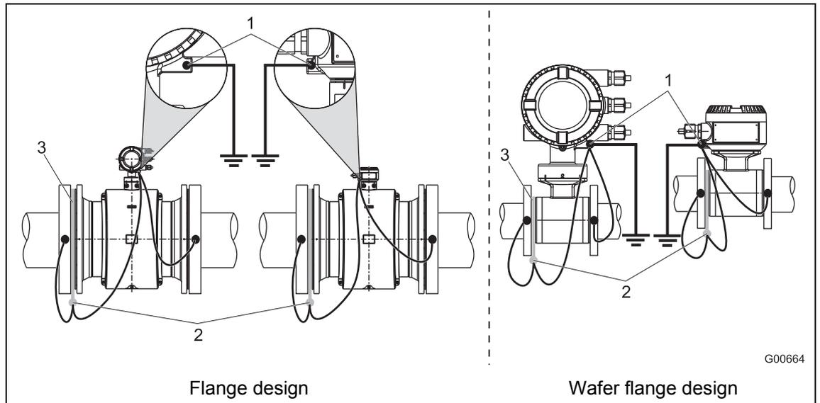
Fig. 27: Plastic pipes, non-metallic pipes or pipes with insulating liner
