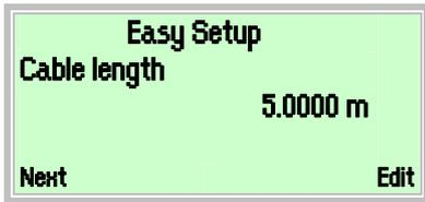
Enter the signal cable length between the transmitter and the flowmeter sensor. For devices with a compact design 0.01 m must be entered.
