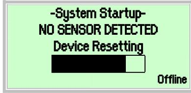
Once the device has been switched on, the sensor calibration data and the transmitter settings are loaded from the SensorMemory into the transmitter. If it is not possible to establish a communication with the SensorMemory<sup>1)</sup>, the shown message appears on the LCD display.
