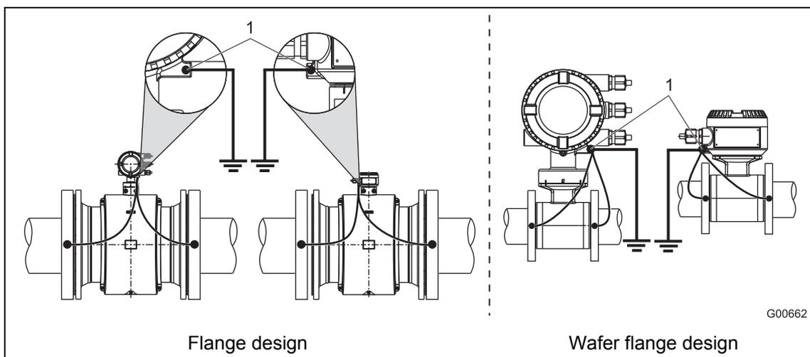
Fig. 25: Metal pipe, without liner
