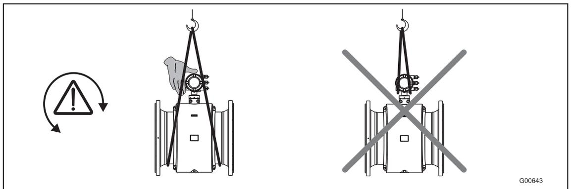
Fig. 7: Transport of flanged units smaller than DN 450
