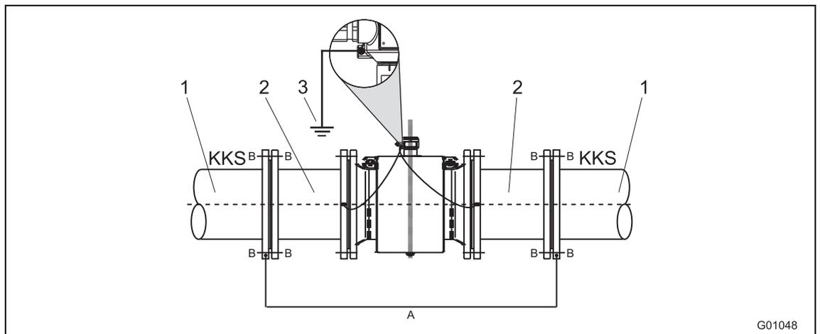
Fig. 31: Flowmeter sensor with functional ground
